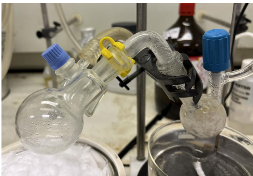
Fig. S20. The set-up of the solid-state depolymerization reaction.
