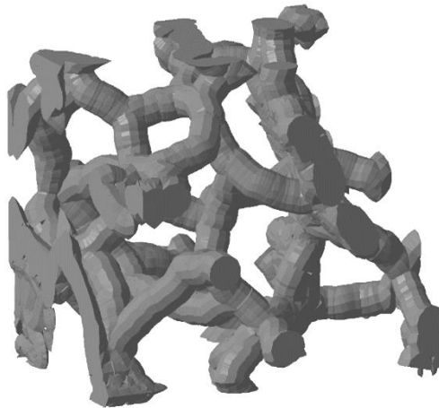
Figure 5.11 Computational image of a bijel template 3D-model architecture with modified solid volume fraction.
