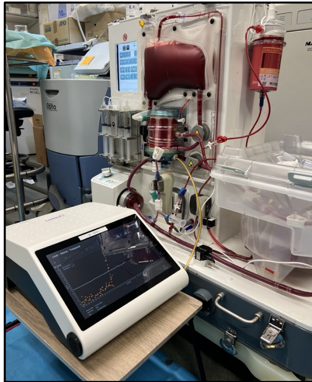
Figure 7.3. The LiMAx FLIP ® 4.0 detection device connected to the CO 2 outlet of the OrganOx metra oxygenator to allow quantification of the 13 CO 2 : 12 CO 2 ratio.
