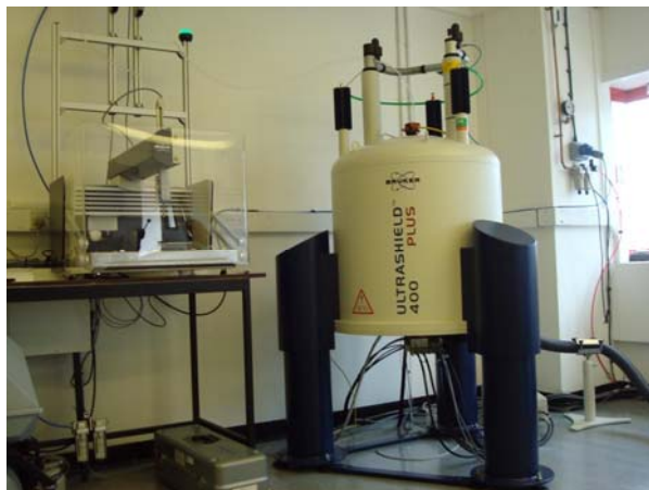
Figure 22: MAS-NMR spectrometer (right) and robotic autosampler (left) in St. Mary's Hospital.
