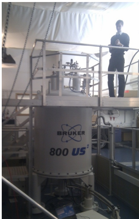
Figure 21: Ryan conducting metabonomics experiments on multiple sclerosis samples using an 800 MHz NMR spectrometer.
