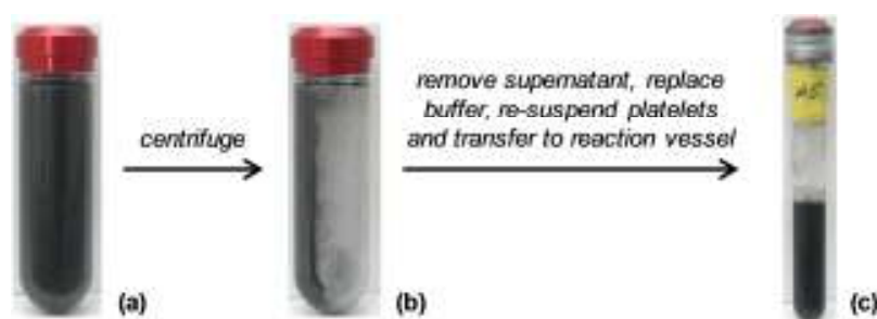
Figure 35 Preparation of the [CODH I -PG-EcHyd2] WGS reaction catalytic system. Photographs of a typical CODH I -PG-EcHyd2 system before (a) and after (b) centrifugation, and following buffer exchange and transfer into a reaction vessel (c). The buffer exchange and re-suspension step was carried out in a glove box under an anaerobic (O 2 < 2 ppm) atmosphere.
