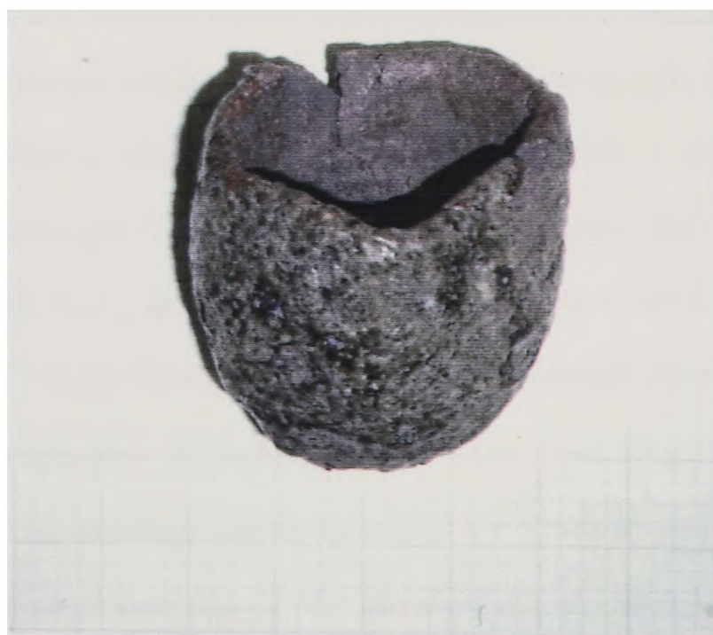
Phot. 12. Crucible from Jakuszowice (hight 35 mm, diameter 40 mm). The XRF of the red 'glaze' on the rim indicated high copper and zinc content.
