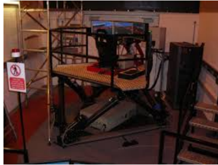
FIGURE 2.2: A smaller hexapod system with simple controls and graphics, installed at the University of Loughborough [25].
