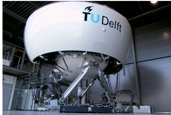
FIGURE 2.1: An example of a typical Stewart platform. This large, high-fidelity hexapod is installed at the Technical University of Delft in the Netherlands [49].
