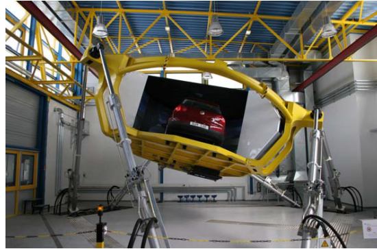
FIGURE 2.3: An inverted hexapod motion platform, at the DLR in Germany [71].
