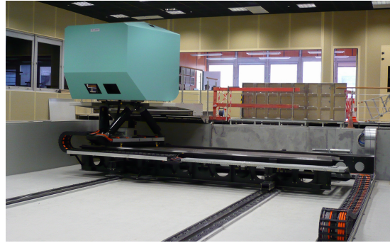
FIGURE 2.4: A graphic reproduction of the Citroen simulator platform with 8 DOF [10]. This is an example of a large workspace, advanced hexapod centred system.
