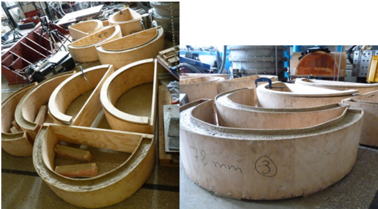
Fig. 5.2. Sample arches cast in timber moulds.
