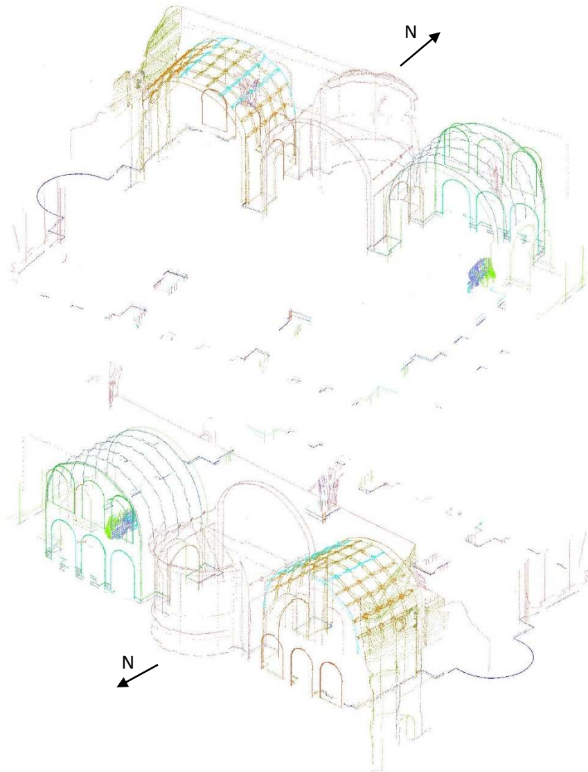
Fig. 2.1. Data points obtained through total station survey of the remains of the Basilica of Maxentius. The different colours signify the different setting out positions of the total station.
