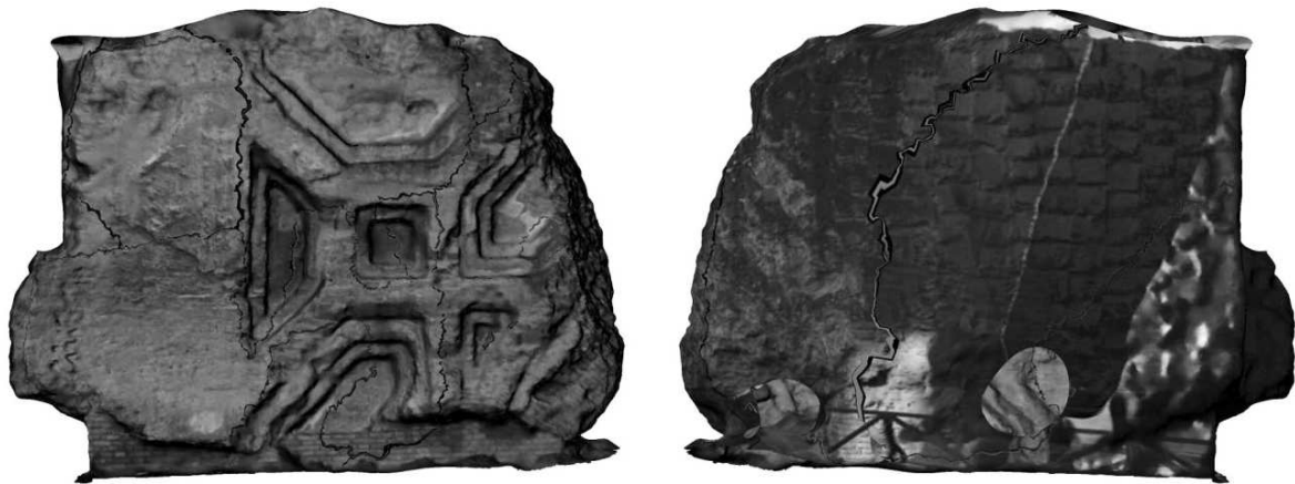
Fig. 2.15. 3D computer model of fragment A generated with photogrammetry software 123D Catch, by Autodesk: view of the intrados (left); view of the extrados (right).
