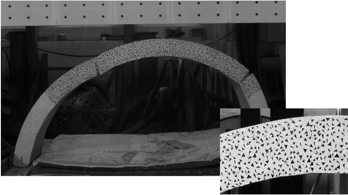
Fig. 5.16. Top left: Example of high speed camera image, at actual resolution, showing static reference points, along the top banner, for photogrammetric rectification and scaling of images. Bottom right: High resolution close up showing pattern devised for PIV tracking, a combination of rectangles of different shapes and sizes.
