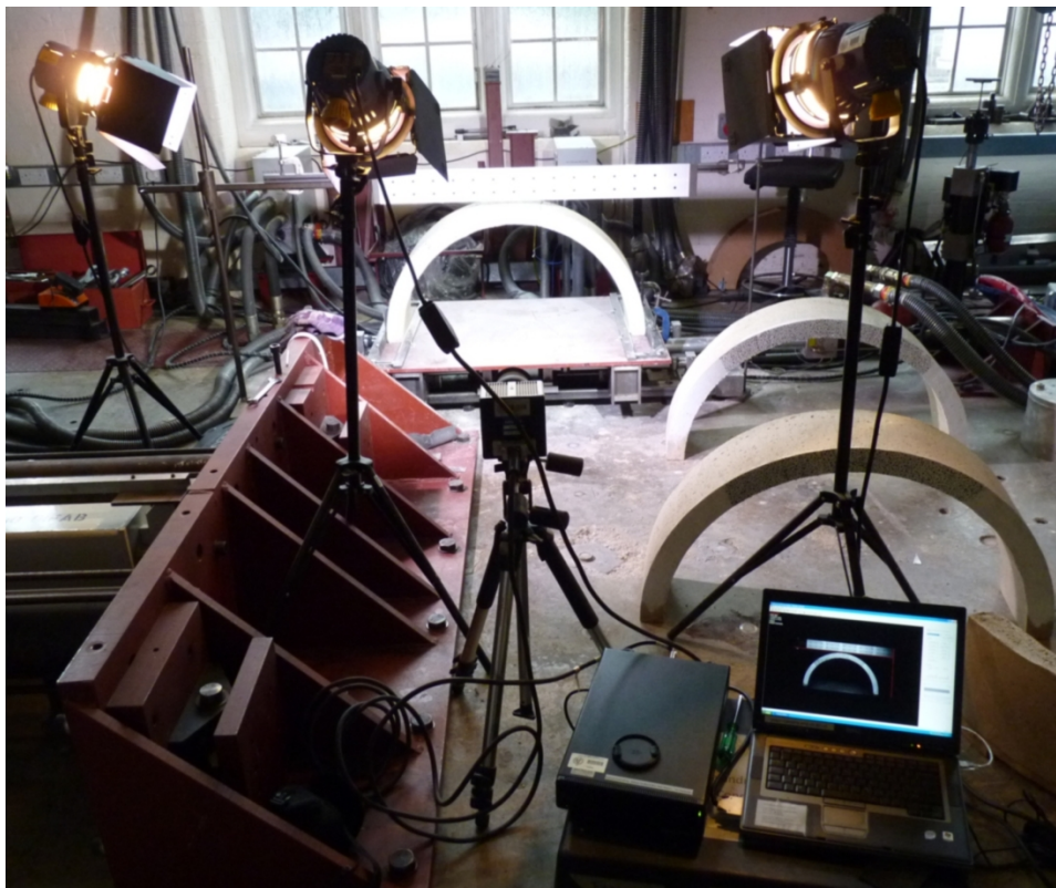
Fig. 5.15. Experimental set-up showing shaking table with arch specimen and high speed camera system.
