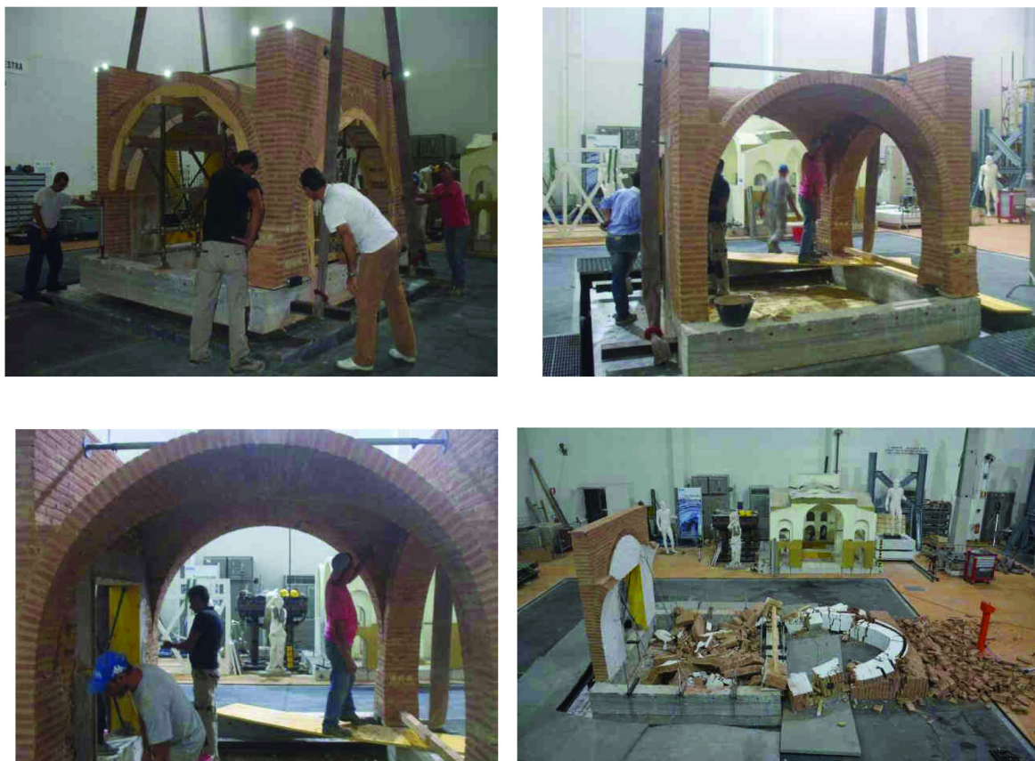
Fig. 4.17. Vault model of the Mosque of Dey (Algiers) constructed in brick masonry: positioning on shaking table and final collapse after testing (PERPETUATE 2012, 81-82).
