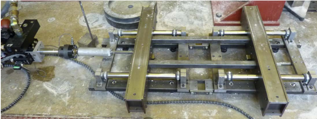
Fig. 5.13. Structure of shaking table: transverse box-section carriages running on linear bearings over cylindrical shafts.
