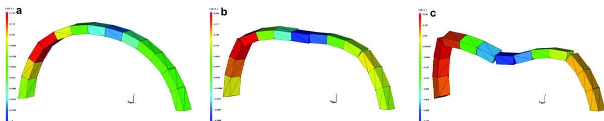
Fig. 4.15. Voussoir arch with dry friction contact subject to seismic loading modelled using LMGC90. Collapse mechanism showing vertical displacements (in m), at times (a) 2.5 s, (b) 2.8 s, and (c) 3 s of the analysis (Rafiee et al. 2008 (a)).
