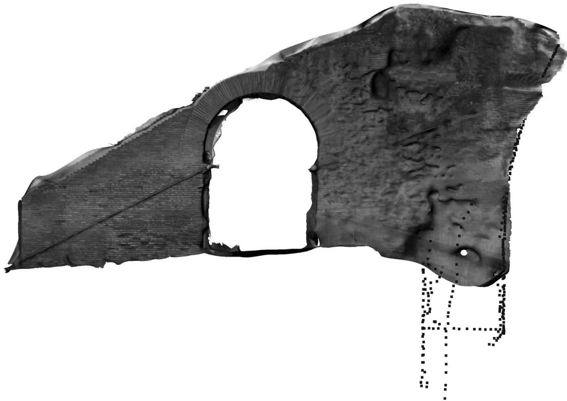
Fig. 2.16. 3D computer model of the roof buttress on axis B, generated with photogrammetry software 123D Catch, by Autodesk: Elevation showing the total-station survey data points used in combination with the 3D model to estimate the level of the lowest point of the roof.
