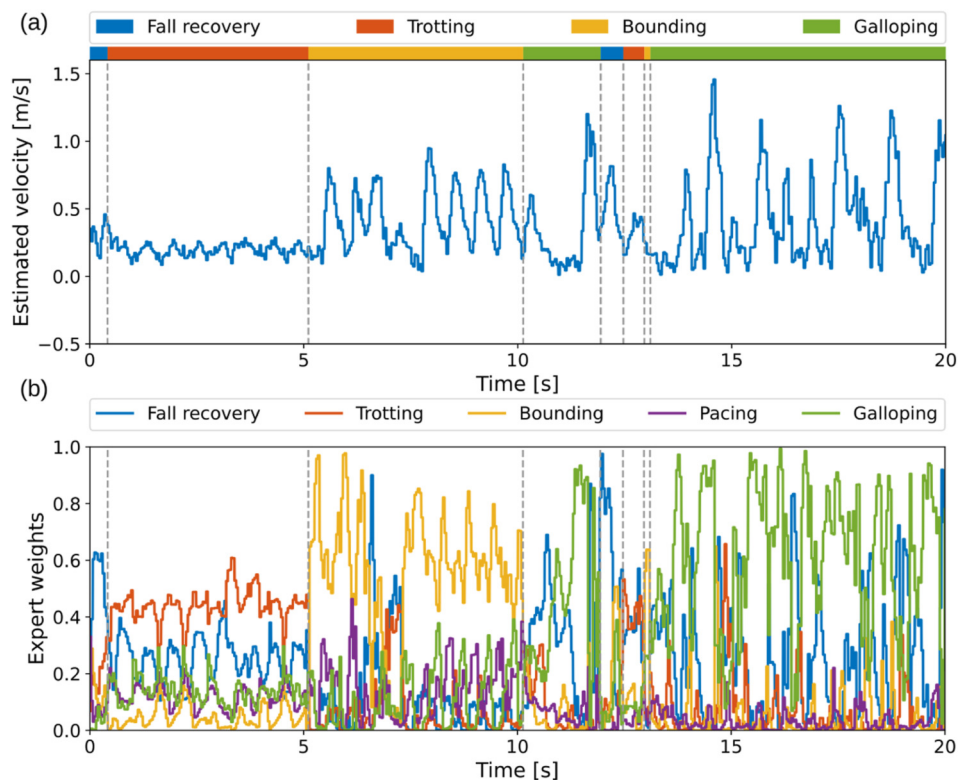
FIGURE 7 Versatile locomotion with continuous gait transitions on the real robot. (a) Estimated horizontal speed of the robot during multi-skill locomotion. (b) Expert weights showing that each motion utilizes all five experts, with one related expert being dominant.
