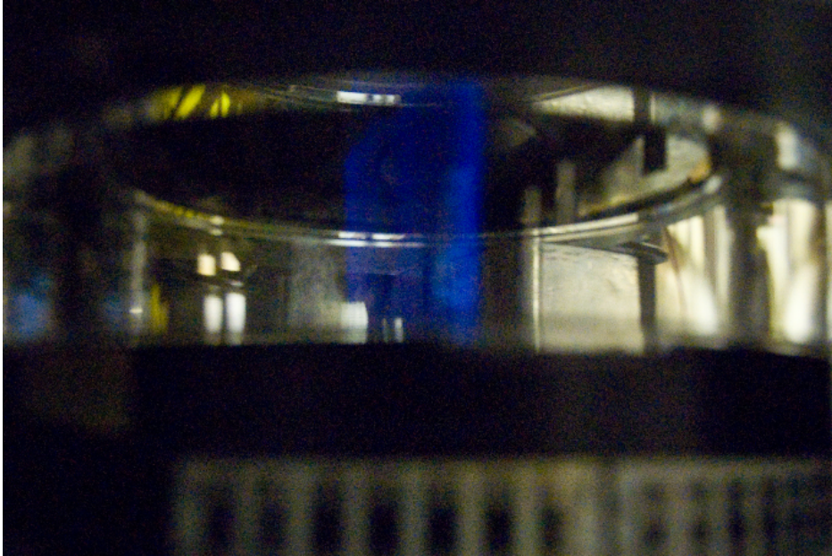
Figure 4.9.: Illustrating the in-cylinder location of the laser sheet with acetone fluorescence.
