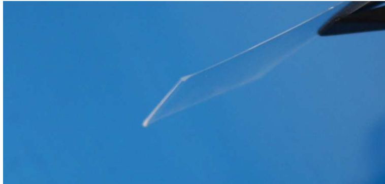
Figure 1.2: Thick edge in a glass sheet redrawn at Schott AG. Photo by Dominic Vella.
