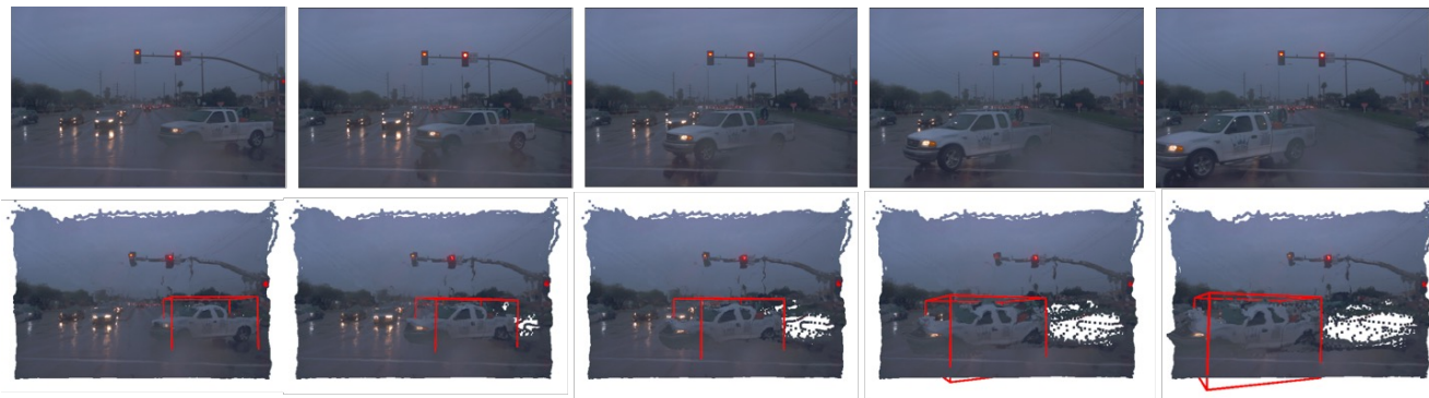
Figure 7. Rigid object motion: 3D bounding box object tracking by masking and aligning the predicted dynamic point clouds.
