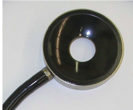
Figure 3.4: Sonic Concepts 483kHz focused HIFU transducer with circular opening for coaxial PCD placement
