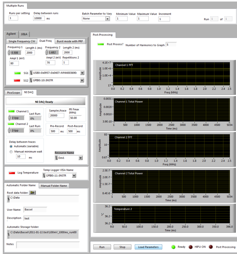
Figure 3.6: Screenshot of the custom-designed LabView interface used to carry out the experiment
