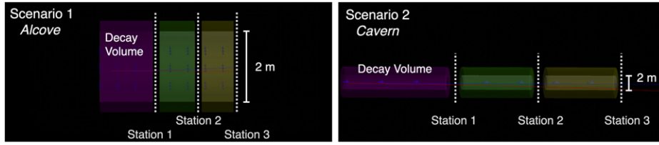
Figure 48. Schematic views of the FASER2 Geant4 simulations for the PPF alcoves (left) and new cavern (right) options. The tracker stations are indicated by vertical dashed lines. For the alcoves design, the tracker stations are 1.5, 2.7, and 3.9 m from the front of the decay volume. For the new cavern design, the stations are 10.0, 15.5, and 21.0 m from the front of the decay volume.
