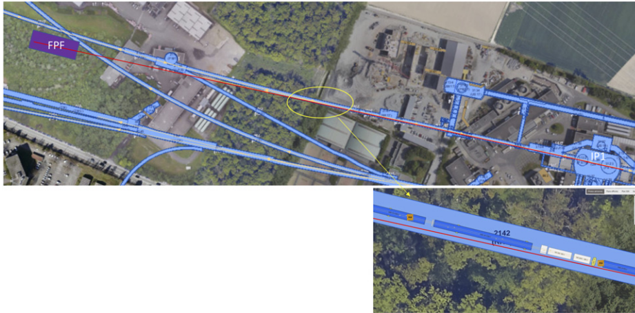
Figure 41. Plan view of the LHC complex between the ATLAS IP and the proposed FPF location. The LOS is shown as a red line, and the region where it has left the LHC magnet cryostats, but remains in the LHC tunnel, is highlighted in the zoomed in region. (Taken from the CERN GIS portal.)
