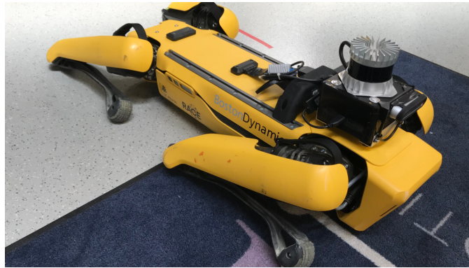
Figure 4.13: The Boston Dynamics Spot robot with a Frontier multi-sensor rig mounted on it. Frontier contains an Ouster LiDAR and an Intel Realsense RGB-D camera. The Spot carries 6 Intel Realsense cameras.
