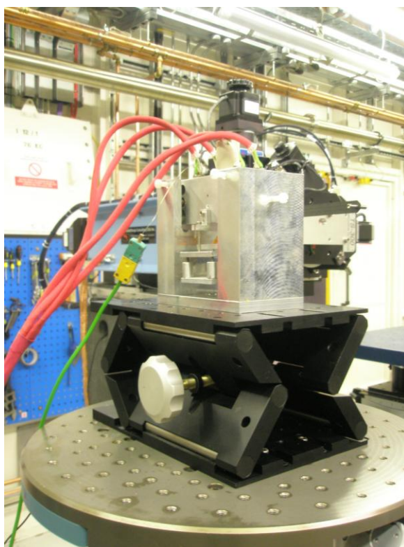
Figure 7.5. An image of a quartz sample stage with temperature controlled block.
