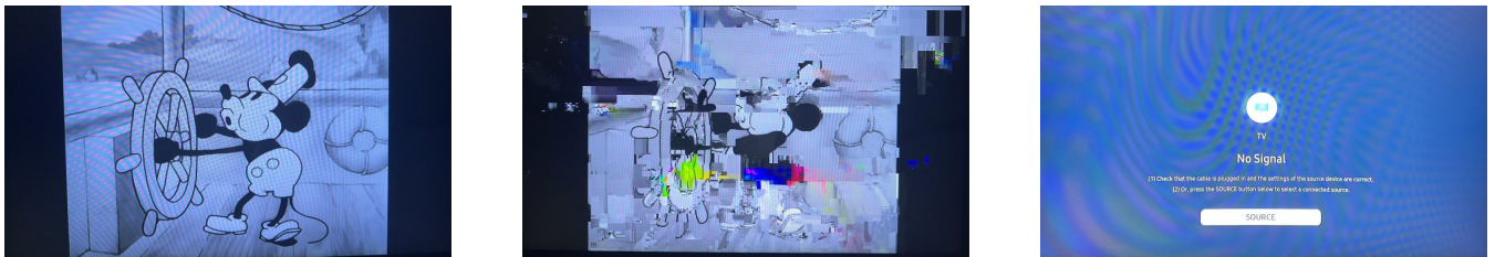
Figure 7: The satellite TV in three states: receiving a clear signal, approaching the limit of signal loss, and signal loss.
