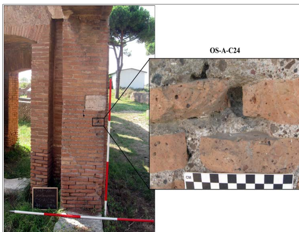
Figure 6.15: Photographs of sampled wall and detail of facing mortar sample (OS-A-C24) location from exterior wall, the facade of the Case a Giardino. Photographs by author.
