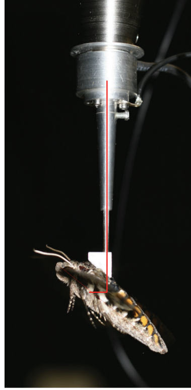
Figure A.3: Once the centre of mass was evaluated, a side-on photograph is used to estimate the distance between the force transducer and the centre of mass for a particular moth.
