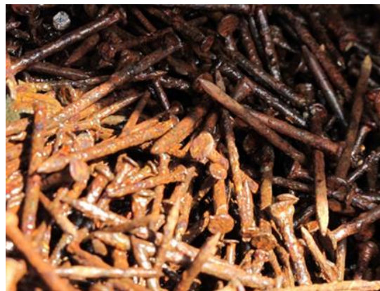
Photo 1.4 Close-up of the ZVI (iron nails)
