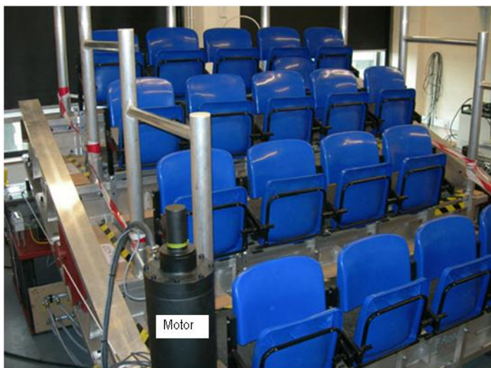
Figure 3.3: Test structure showing one of four motors located on each corner (Comer et al. 2010)
