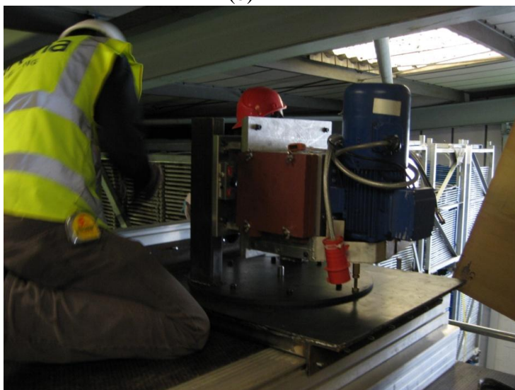
Figure 7.16: (a) Exciter mounting assembly (b) Attaching the eccentric mass shaker to the test structure
