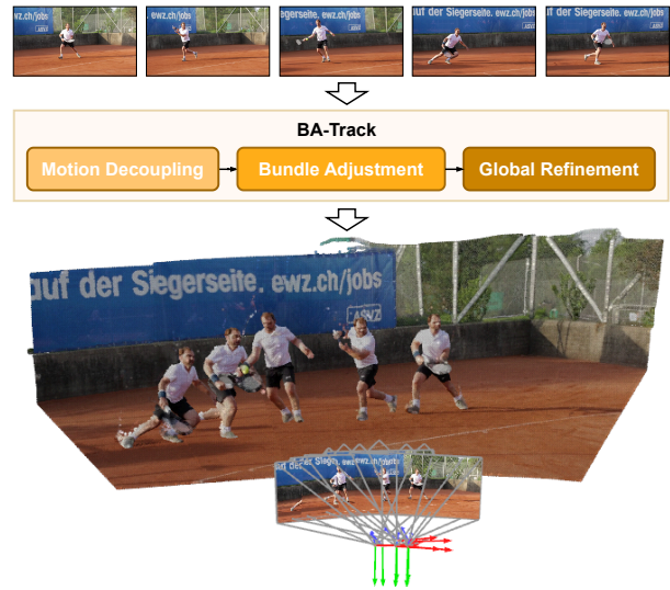
Figure 1. Framework preview. Given a casual input video, BA-Track uses a 3D tracker to separate camera-induced motion from the total observed motion, enabling bundle adjustment to process both static and dynamic points. Using the aligned sparse point tracks from bundle adjustment, we refine the dense depth maps, producing a globally consistent dynamic scene reconstruction.
