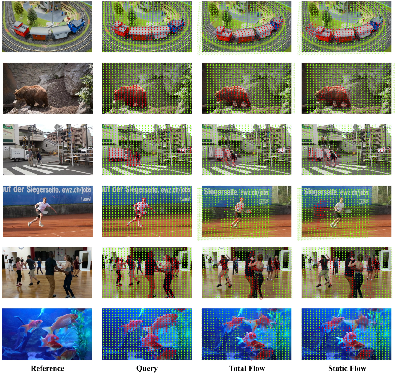
Figure 10. Visualization of motion decoupling on the DAVIS dataset [21] . The reference frame corresponds to the first frame of the video, from which the queries are extracted. The total flow represents the combined motion of points, while the static flow refers to the motion attributed solely to its static components. The estimated static and dynamic trajectories are depicted in green and red, respectively. We observe that the red points in the static flow largely remain in their original reference frame, signifying successful motion decoupling.
