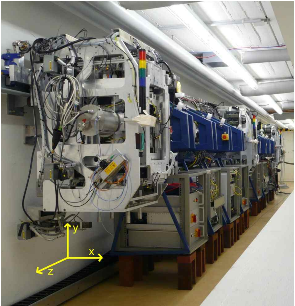
Figure 3.6: View down the train from the left hand side of car 1, dominated by the motor cage framework, The circular launch end-cap can clearly be seen, connected to the the 57FCM infra-red LSM laser by the blue fibre-optic cable. The pillar of lights is used to alert users to the current status of the train, warning them of car alignment or train motion. The bricks supporting the support crates are a temporary installation as part of a stability experiment. The general directions of the lab axis system are shown.
