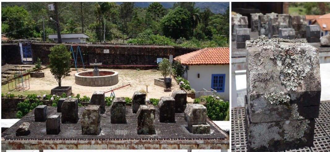
Figure 4 Examples for simpler blocks (compared to the Asterixe) exposed in Brazil as part of the IDEAS project (source: E. Wendler).
