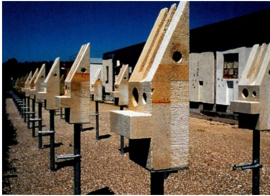
Figure 1 Germany, Holzkirchen, test site with 'Asterixe' specimen (Snethlage 2005, p77).
