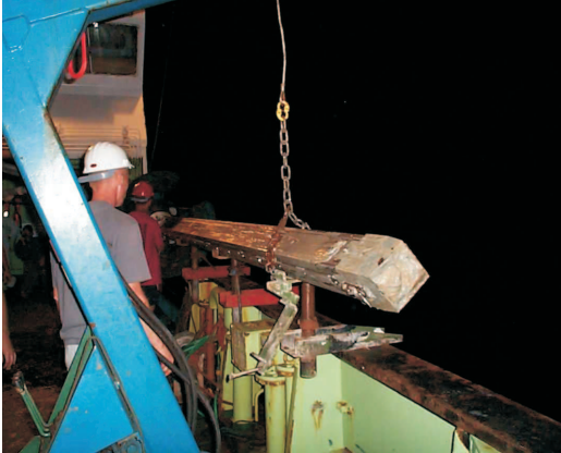
Figure 2.3: A Kasten core being recovered aboard RRS Charles Darwin .
