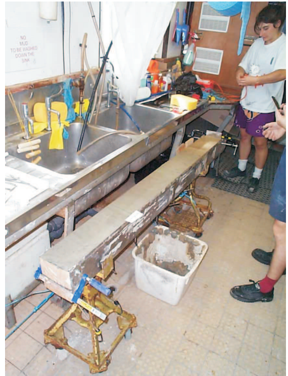
Figure 2.4: A Kasten core with the upper 'side' removed exposing the sediment. The screws for jacking up the false bottom are visible protruding from the underside of the core.
