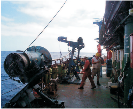
Figure 2.5: A piston core being recovered aboard RRS Charles Darwin . This core bent while penetrating the sediment.
