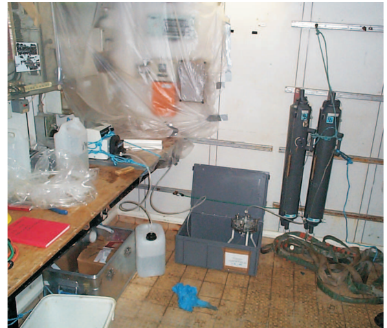
Figure 2.2: The “Wet Lab” aboard the RRS Charles Darwin with the filtration apparatus. The set up is such that water is filtered directly from the Niskin bottle, through the filter, under suction provided by a peristaltic pump. The filtered water passes directly into the sample bottle through a specially modified cap so the sample’s contact with the air and hence contamination from the lab is minimised.
