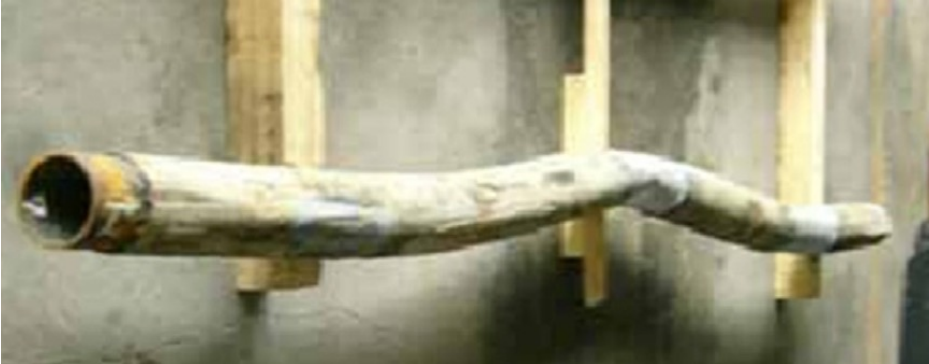
Figure 1.1 Pipeline buckles in vertical direction (Upheaval Buckle), Mitsuya 2013
