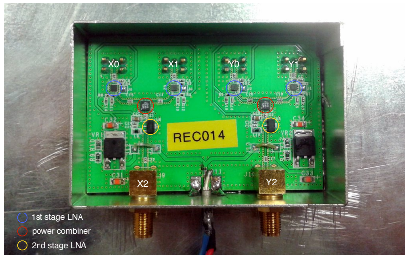
Figure 3.11: D-PAD receiver board. Input pairs (X0, X1) and (Y0, Y1) are amplified, power combined, then further amplified, before being output on X2, and Y2 respectively.
