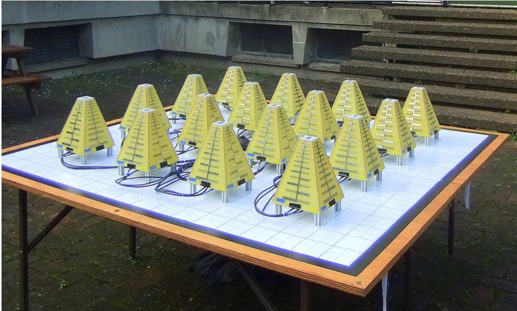
(a) D-PAD single station in 4 \times 4 square configuration
