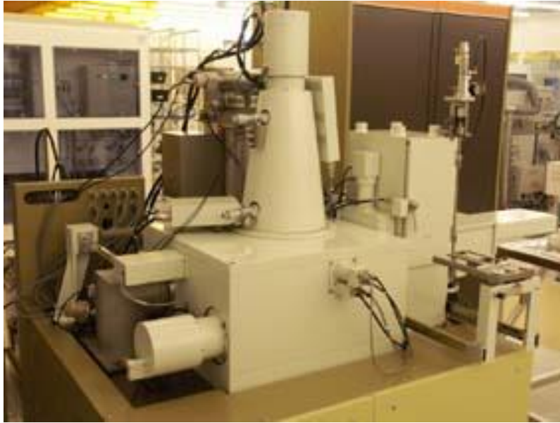
Figure 2.3. JEOL JBX-5DII e-beam machine, photo of the Main Console [66].
