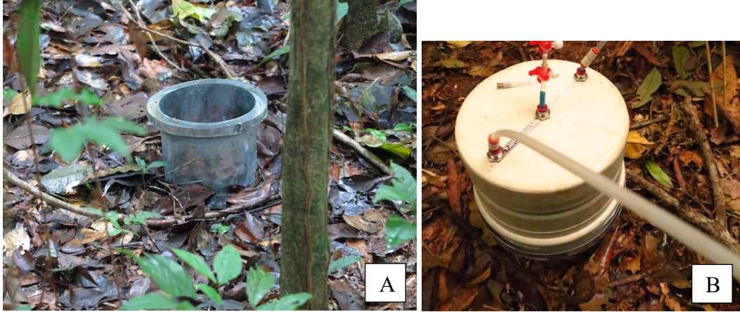
Supp. Methods Fig 2. Gas sampling ring (A) without and (B) with the gas sampling cover mounted on top of it.
