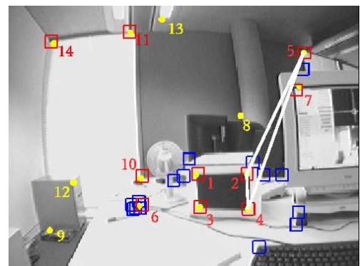
(c) A set of three potential matches (joined by white triangle) is selected and the three-point-pose algorithm is used to give a camera pose hypothesis. The other map landmarks are then projected into the image (yellow circles) using this pose and the metric map. The high consensus of seven matched projections shows this pose is correct.
