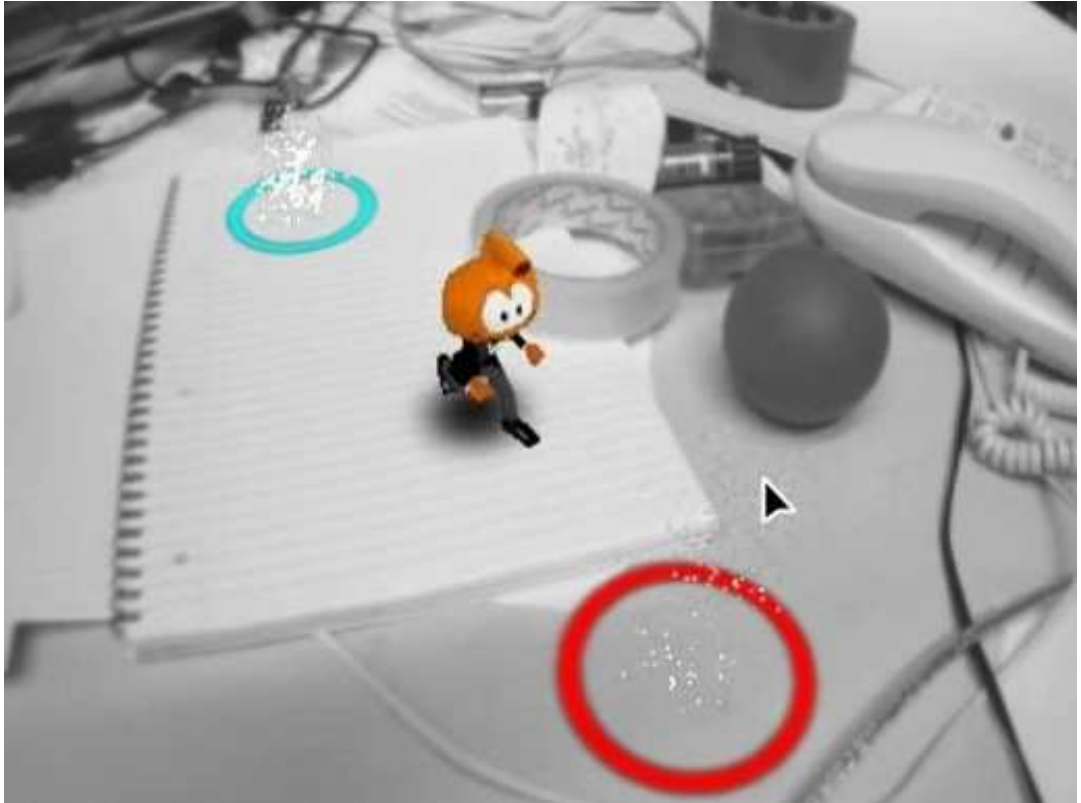
Figure 1.2: Augmented Reality: An important application for monocular SLAM is augmented reality. This technique allows virtual objects to be added to live video using the pose of the camera relative to real objects in the world. Since our system provides the relative camera pose as each new frame arrives, the virtual character in this computer game (shown in colour) can be rendered on live video to make it appear to be running across on the real desk (shown in greyscale). The user is able to move the camera around the scene to view the virtual objects in the real setting from different angles.
