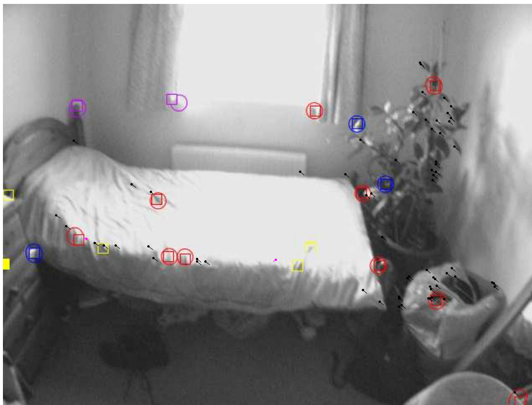
Figure 3.2: Monocular SLAM with Visual Odometry: While tracking the ordinary map landmarks, up to 200 visual odometry features can be used to refine the estimate of the inter-frame motion. The black lines here show the visual odometry features motion from position in the previous frame ( \bullet ). Two observations have been rejected as outliers and are shown in magenta (one of these is easy to find in the centre of the image). The observed map landmarks are shown in red if the measurement was successful, blue when no match was found, and magenta if the observation was rejected by JCBB. Ellipses indicate the active search region. Landmarks not selected for observation in this frame are yellow . The 3D state estimate at this timestep can be seen in Figure 3.4.
