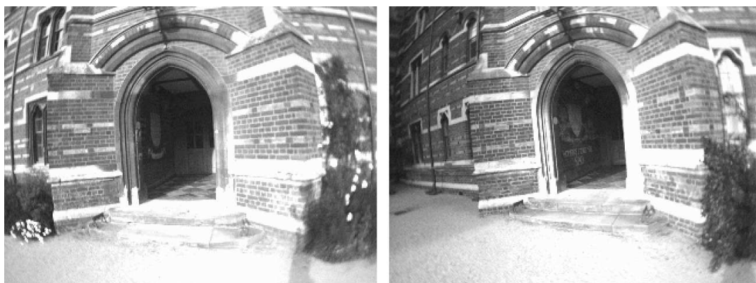
Figure 5.16: Despite these two regions of the world having both similar appearance and structure, they belong to different parts of Keble College courtyard. A loop closure detection system should indicate a match and a higher level system should then be used to mark it as false using either the uncertainties in the global metric map or more observations before and after the archway.
