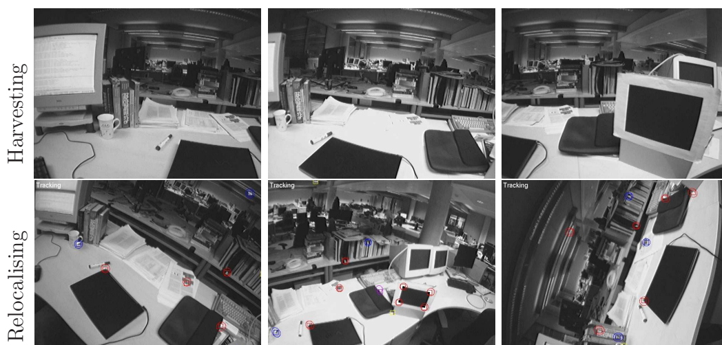
Figure 4.13: Relocalisation from Novel Views: Here tracking (and thus harvesting) was only performed along a short linear motion illustrated by the top row of images. This is sufficient to allow relocalisation from the views shown in the bottom row despite the difference in viewpoints. A metric representation of this experiment is shown in Figure 4.12.
