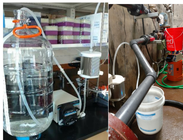
Fig. 35 UV LED reactor disinfection performance was assessed under varying conditions at bench scale (left) to develop a predictive model that was used to assess performance during challenge testing after pilot installation (right).
