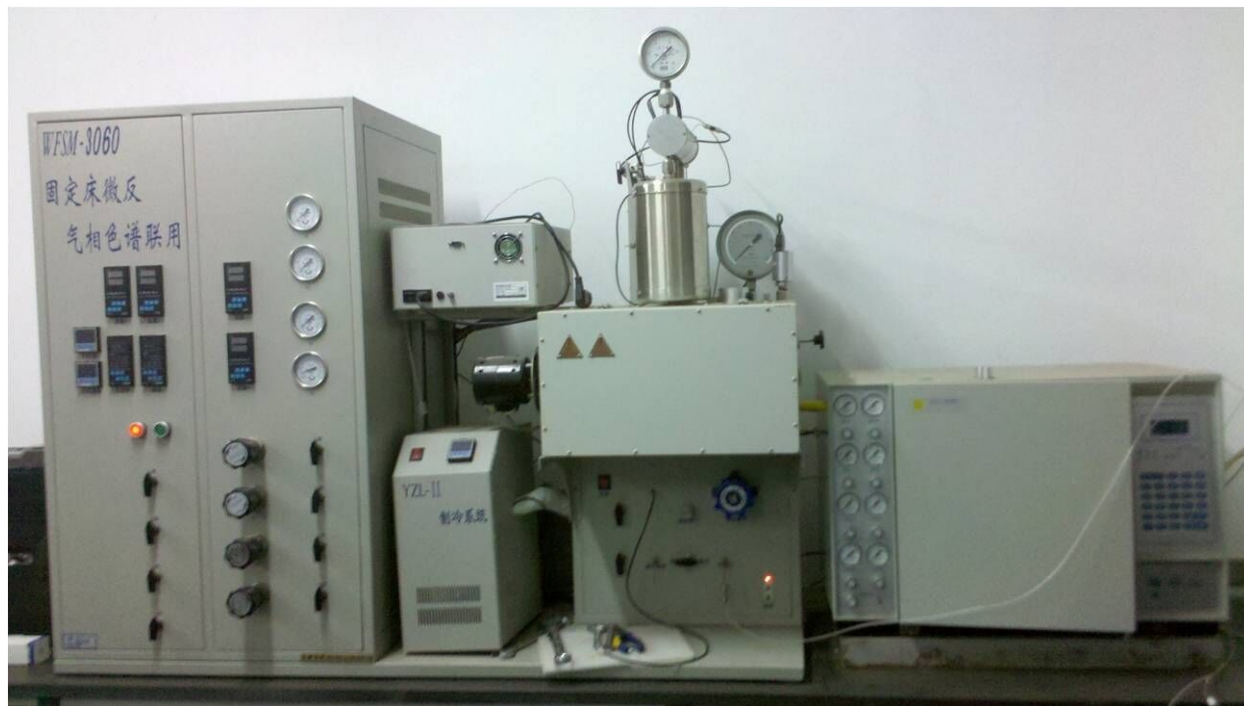
Figure 3-1 The employed fixed bed micro-reactor for CO 2 hydrogenation at Wuhan University, Wuhan, China
