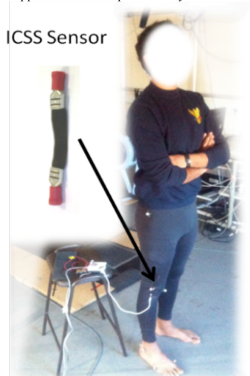
Figure 5-10. A subject wearing the ICSS garment and optical tracking markers
