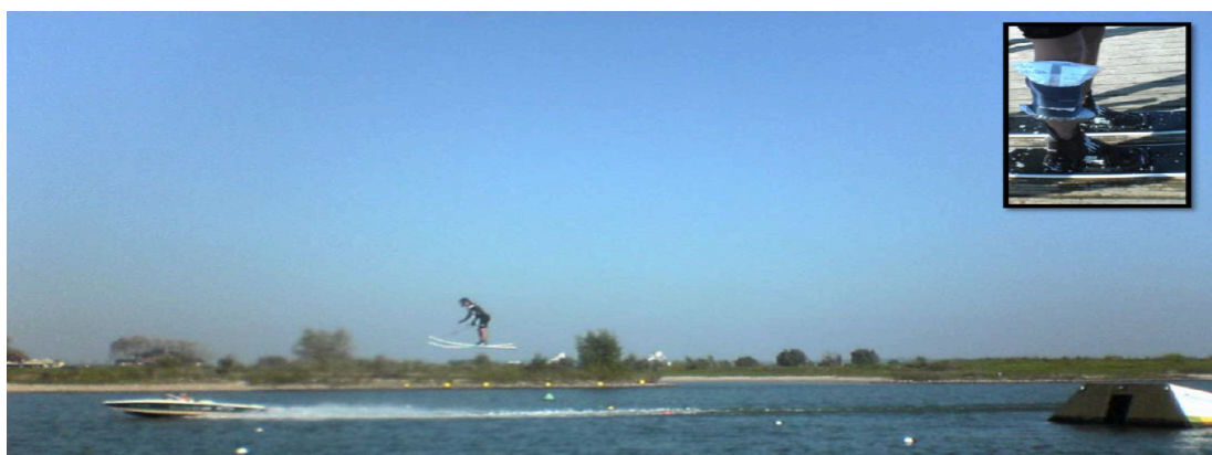
Figure 5-1. Water-ski jump performed by participant. Inset picture shows the placement of the waterproofed accelerometer and datalogger.
