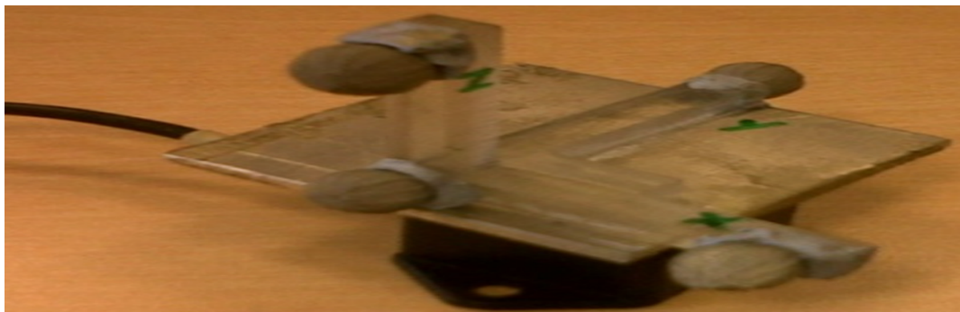
Figure 5-4 Marker cluster placed on the wired accelerometer. The markers were used for the construction of a local coordinate frame
