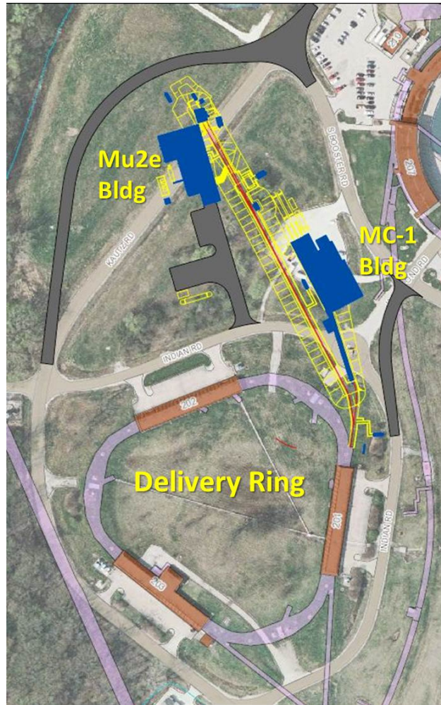
Figure 7.48: Tunnel enclosures and service buildings for the Delivery Ring, M4 and M5 lines, and experiments
