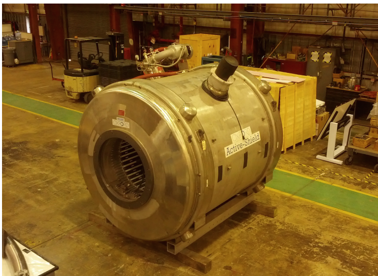
Figure 15.17: The 4T, test solenoid OR66 from Oxford Instruments inside building 366 at Argonne National Laboratory waiting for installation.
