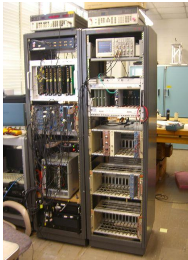
Figure 21.4: Photograph of the DAQ test stand including \mu TCA-based electronics and VME-based electronics at UKy.
