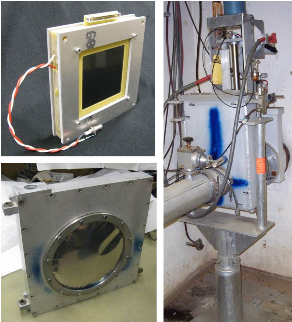
Figure 7.84: The first completed PWC prototype (top left). The signal connection is at the top and the high voltage connection comes out the left side. The PWC is installed in an anti-vacuum box (lower left). ArCO 2 gas is pumped into this chamber, and there is a vacuum window on both front and back of this module. The anti-vacuum chamber is installed inside of the bayonet can (right) which is pumped down to beam tube vacuum. The PWC wires can be lowered into the beam or raised out of the beam via a motor drive.
