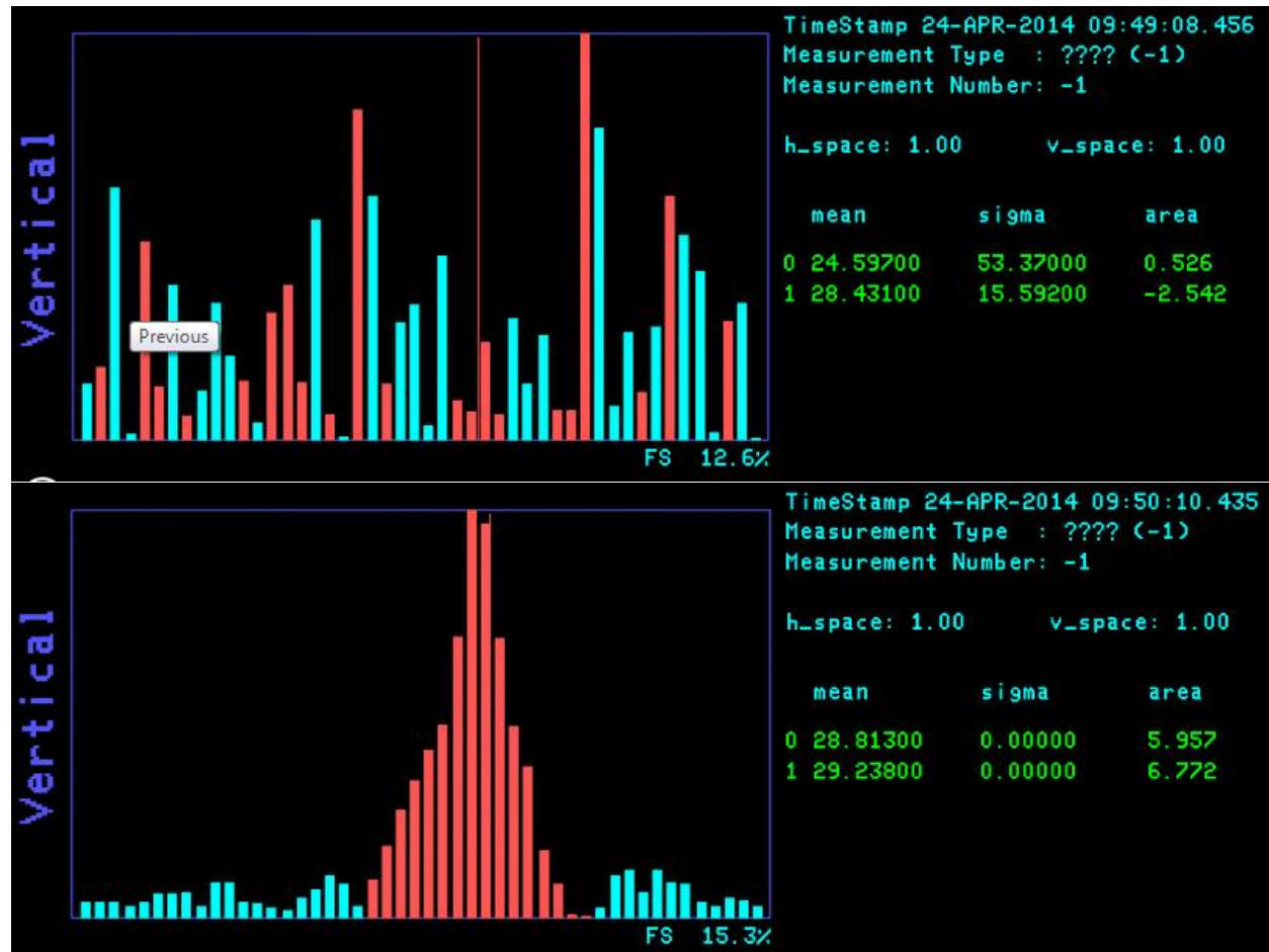
Figure 7.80: Wire profile at the 728 location for 10^{11} 120-GeV protons on target with 2.5 \times 10^8 low-intensity secondary beam measured using an ion chamber at at 728. The top plot is the noise sample and the bottom plot shows the results of subtracting the noise sample from the raw beam signal.
