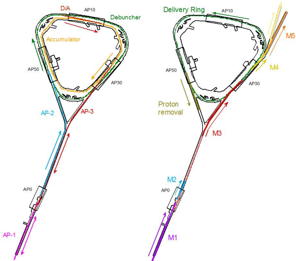
Figure 7.25: Layout of the Antiproton Source beamlines (left) and the reconfigured beamlines for (g - 2) operation (right).
