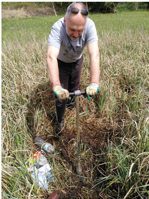
FIGURE 2.12. Taking peat/sediment samples using a Russian corer at Daisy Banks Fen, Oxfordshire (Photo: E. Forster).
