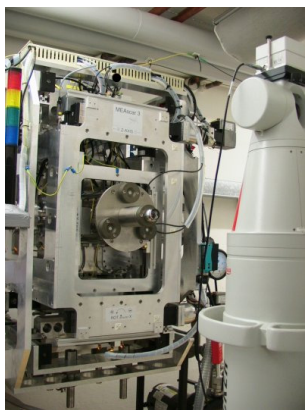
Figure 1: Laser tracker assisted calibration setup of the RTRS in the DESY test tunnel (June 2008)
