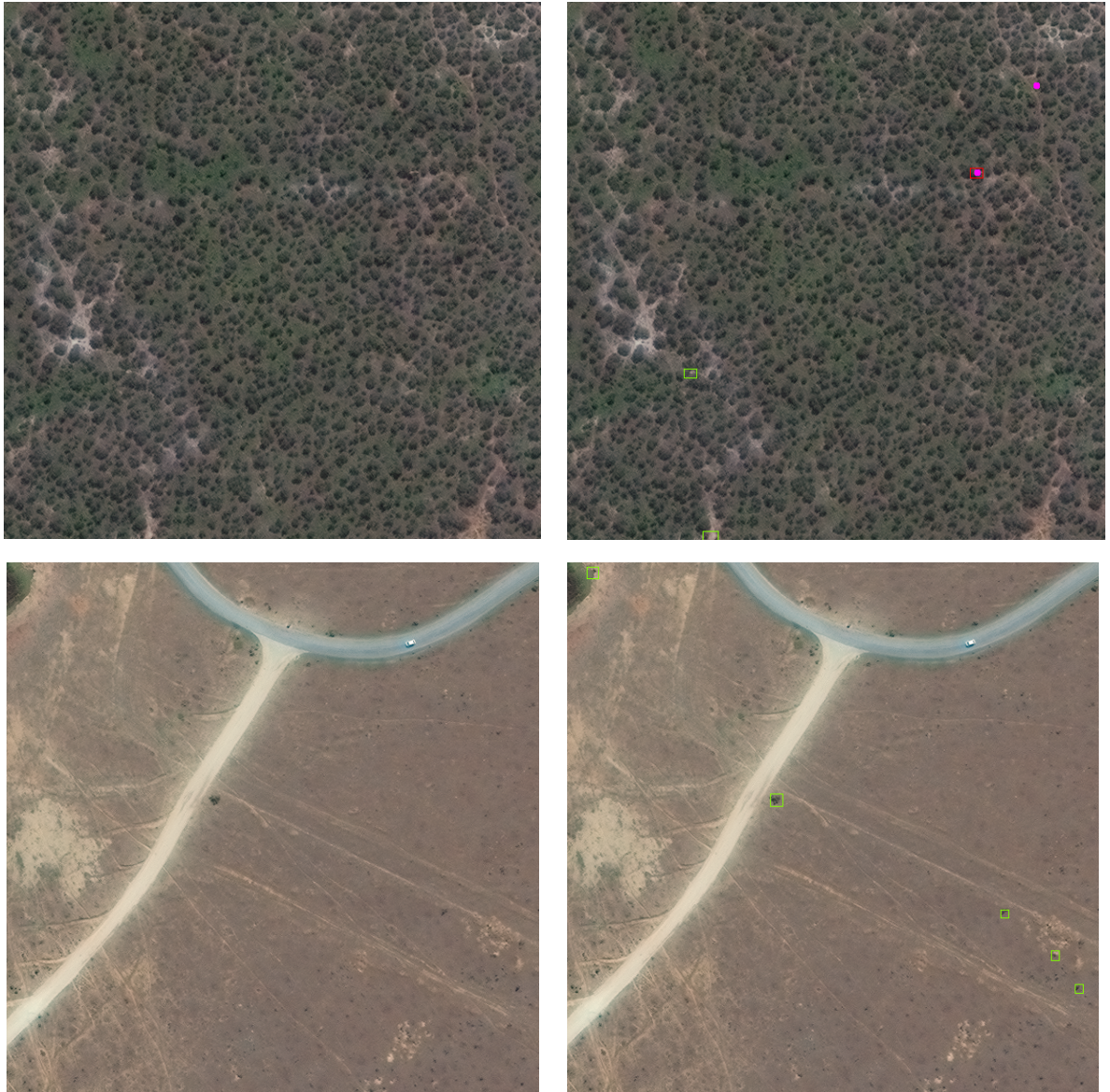
Figure 2 Sample showing human and CNN detections where the humans outperform CNN models. CNN detections are (green boxes) and ground truth labels (red boxes) and human labels (magenta circles). Raw images on left, detections on right. Satellite image (c) 2020 Maxar Technologies
