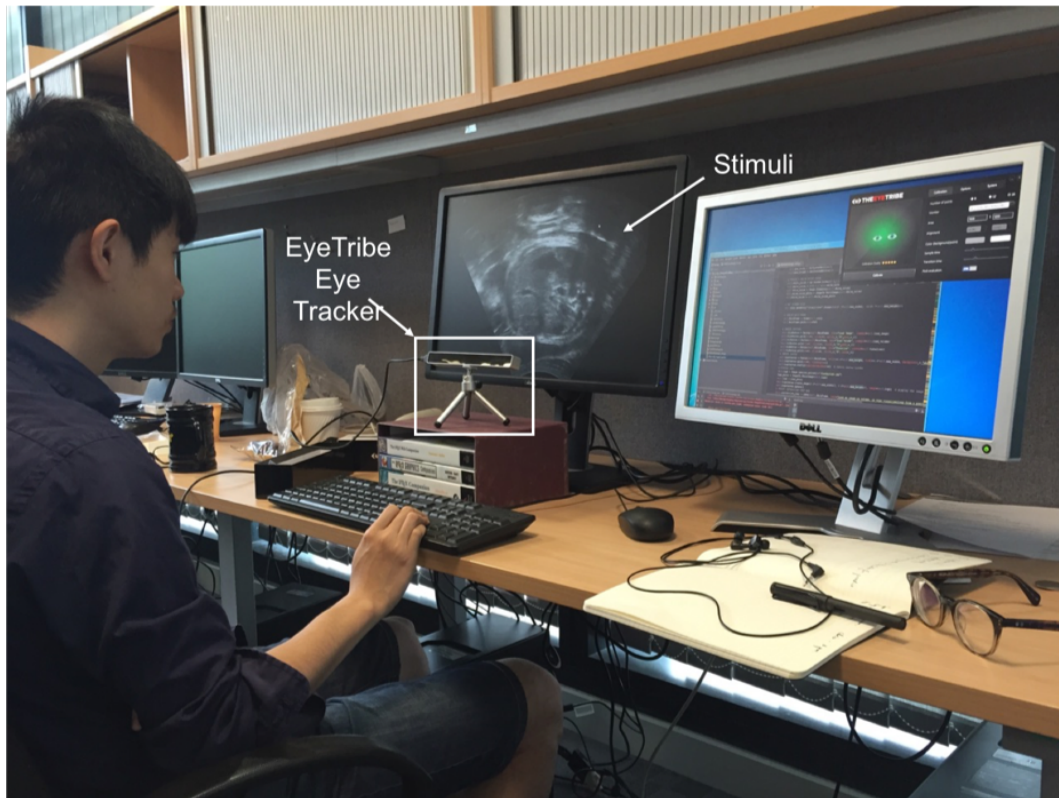
Figure 4.3: The experimental setup of gaze-tracking experiment on fetal abdominal US videos, consisting of a screen that displays stimuli, an eye-tracking device, and a keyboard for navigation through ultrasound frames.
