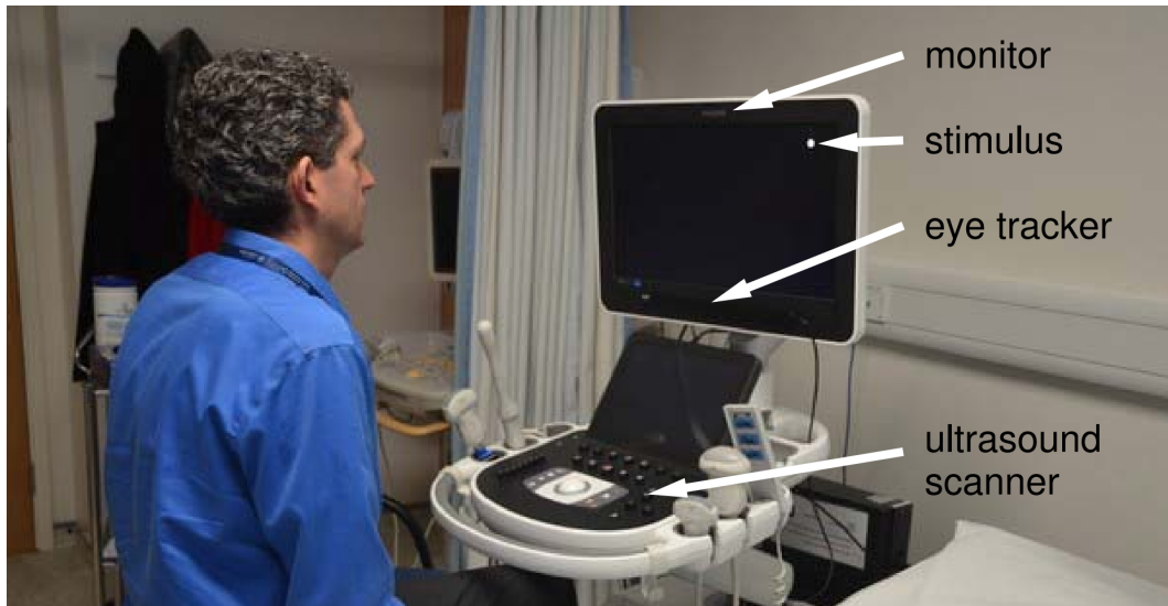
Figure 6.1: The experimental setup of gaze tracking experiment of PULSE project, consisting of a screen that displays stimuli, an Tobii eye tracker attached to the bottom of a monitor, and a GE Voluson E8 scanner. The figure was reproduced from [chatelain2018evaluation] ©IEEE.
