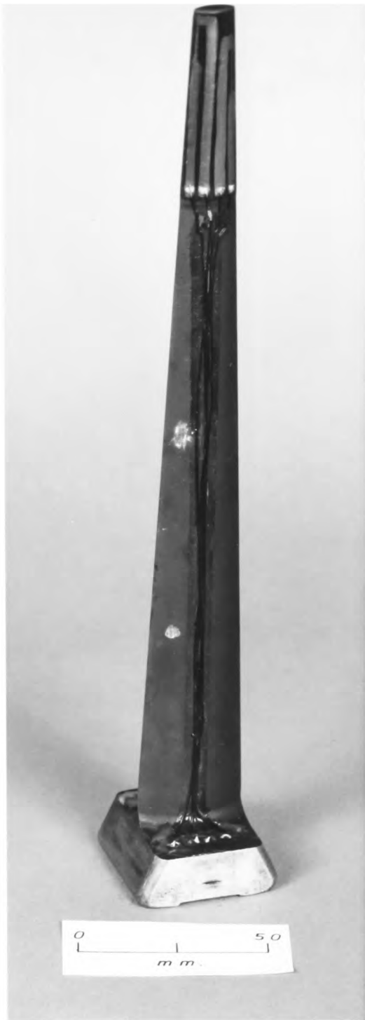
Figure 5.15: Bar from Spinning Rig Instrumented with Thin Film Gauges.
