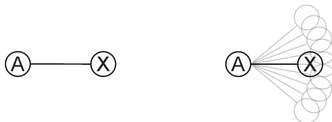
Figure 2.14: A sketch to indicate how bending bonds may appear shorter in diffraction experiments (right) than in calculations (left).
