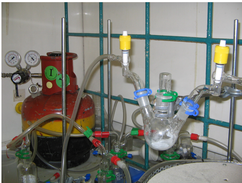
Figure 2.2: The apparatus used for single-crystal growth, showing a reaction between \text{LiBH}_4 and \text{NH}_3
