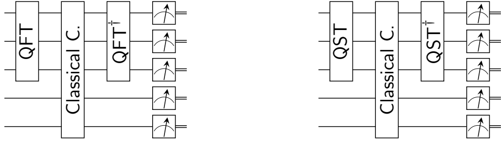
(a) Quantum circuit used in Shor’s factoring algorithm [8]. The classical circuits between the transforms represent a polynomially-long sequence of Toffoli gates.
