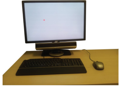
Fig. 7. Our experimental setup consists of an SMI RED500 gazetracker that determines the user's gaze position on a 24-inch screen with a 1920x1200 resolution.
