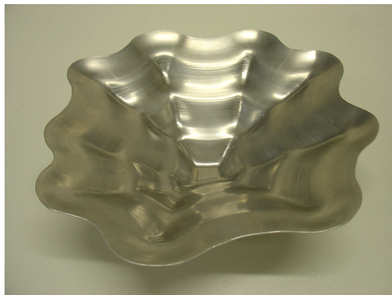
Figure 1.5: Asymmetric part formed on the Cambridge ISF machine.
