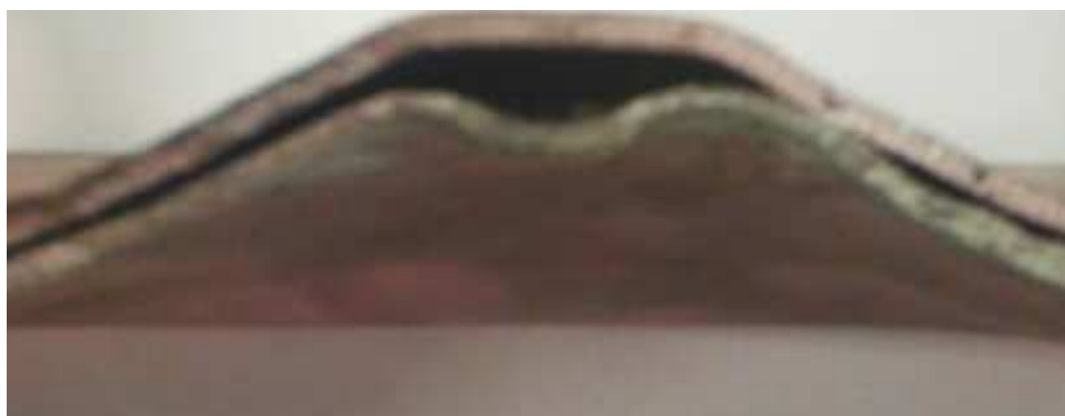
Figure 3.35: Cross section through incrementally formed pure copper (top) and annealed copper (bottom). Both specimens are 0.25 in thick and were subjected to the same tool-path.
