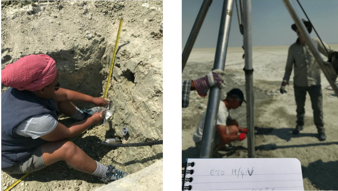
Figure 3.1: Photographs of fieldwork in Etosha. Left: OSL Sample collection from a site on the lakebed (Credit: A. Nagendji). Right = Photograph of vibracorer during sample collection of Core B (ETO 19-4V).
