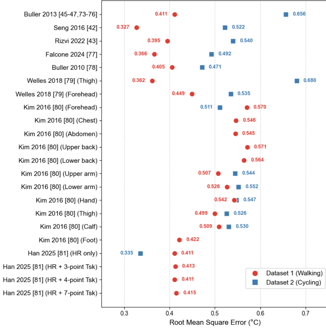
Figure 3.5: Benchmark comparison of continuous core body temperature tracking accuracy of selected studies, quantified by RMSE.
