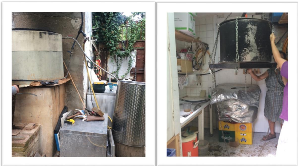
Figure 6.3. a) The ‘beer factory’ with rocket stove (left) and b) the mash tun lifted up (right). Source: Author
