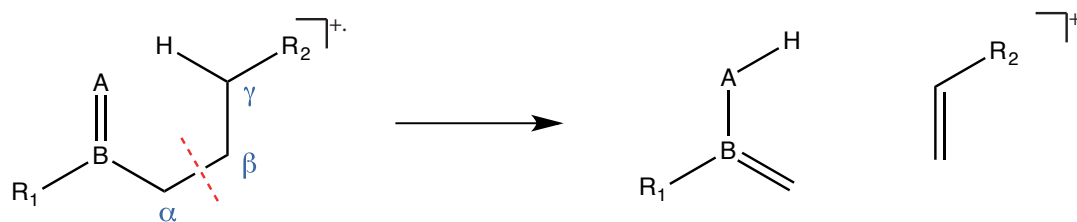
Figure 7.1: The McLafferty rearrangement, which proceeds with transfer of a \gamma -hydrogen atom through a six-membered transition state to a double bonded atom and results in \beta -bond cleavage.
