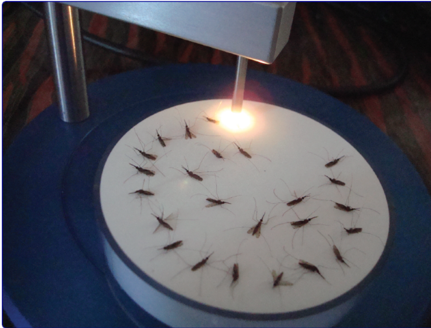
Figure 4.1: A near-infrared spectroscopy machine being used to scan individual mosquito samples. Image adapted from Sikulu et al., 2011.
