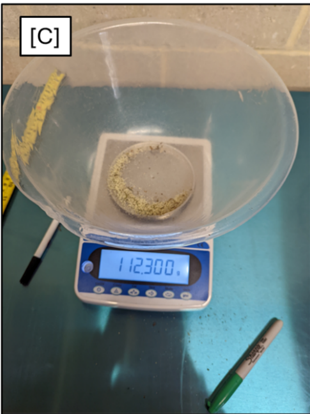
Figure 3.5: Laboratory measurements and processes of destructively sampled scrub trees [A] processed samples in paper bags ready for oven drying; [B] size categorisation of root classes based on diameter; [C] precision balance scales used to weigh samples, including the excess saw dust created during the processing (displayed here); [D] digital crane scale used to weigh the total weight of the scrub tree.
