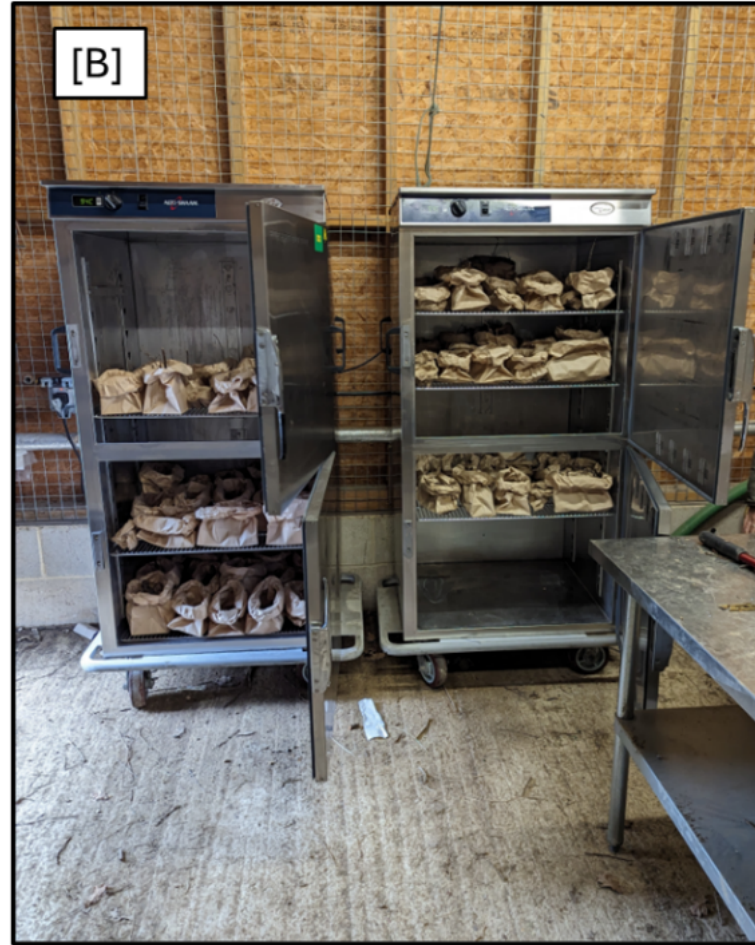
Figure 3.4: Destructive sampling process in the field and in the laboratory [A] combination of the mini digger and the compressed air to extract a scrub tree; [B] samples in paper bags in ovens; [C] trench dug 0.5 m deep to extract the root ball of a larger tree.
