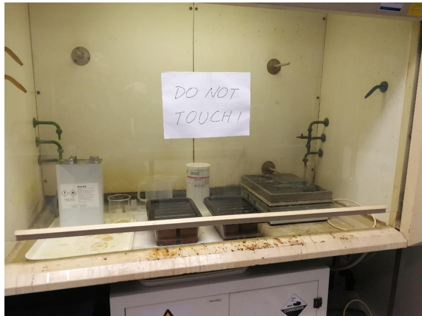
Figure 3.7 Samples in sealed consolidant bath stored in ventilated fume cupboard at Geolabs facility. Image © Author
