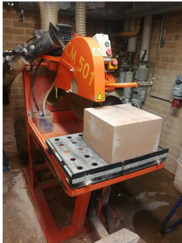
Figure 3.4 Norton Clipper saw at Geolabs Facility, with Locharbriggs sample pre-cutting, image © Author
