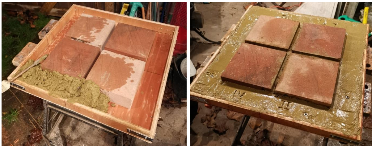
Figure 3.5 Construction of the Pedatron Foot Erosion Platform, Image © Author
