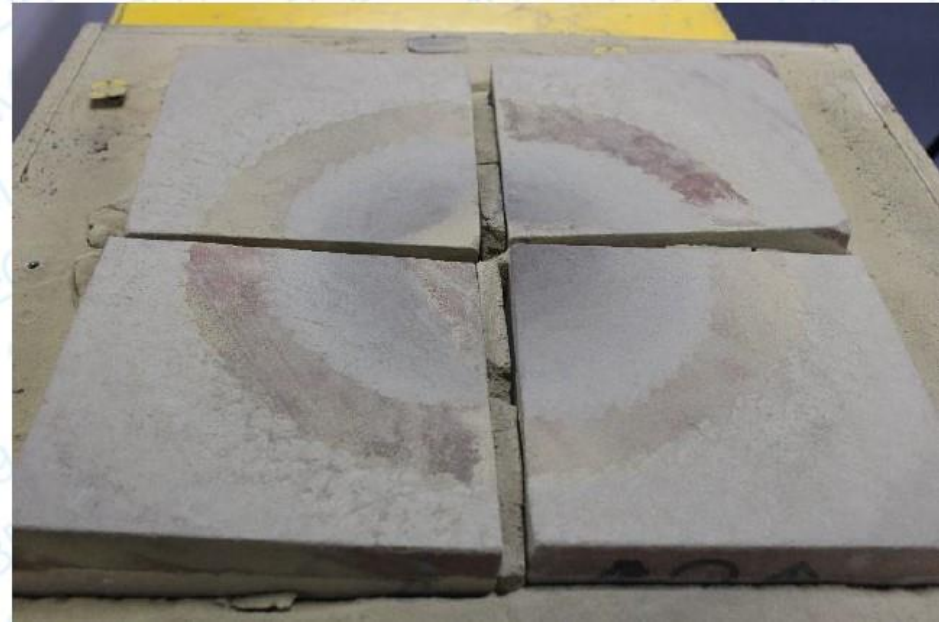
Figure 6.10 Walking Platform immediately post- first test, pre-cleaning. The 'doughnut' effect is clearly visible as a circle spanning the four tiles. Also clear is the movement of the tiles within the frame. Image © SATRA
