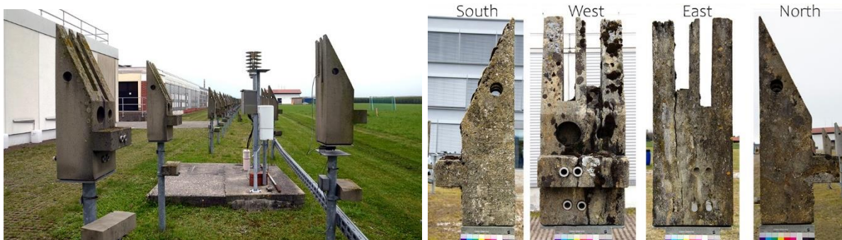
Figure 1.4 "Asterixe" test pieces on site in Holzkirchen, Germany. Images ©K Wilhelm
