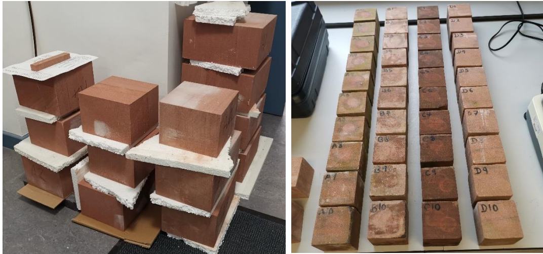
Figure 3.3 Left: Stone for test wall during cutting, at Geolabs, Right: Sample blocks for exposure rack trial following experiment. Note darker shade of Weathered and Untreated samples (2 nd from right). Images © Author
