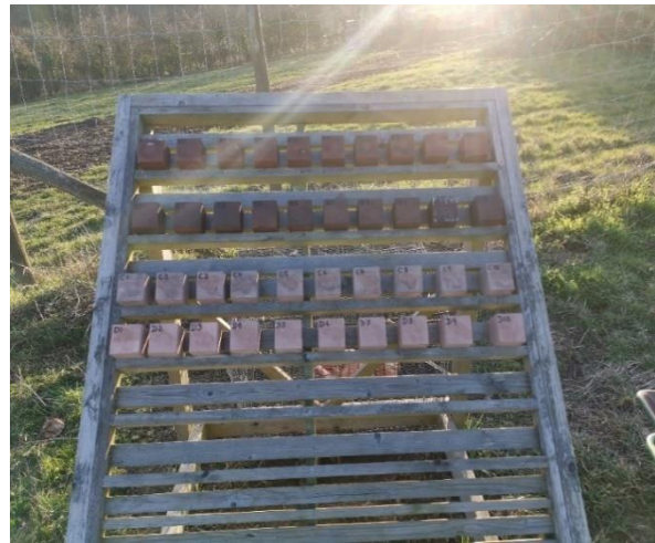
Samples arranged in rows per treatment: Top: TEOS treated, Second Row: MTMOS treated, Third row: Weathered and Untreated, Bottom Row: Natural condition
